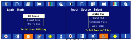
Push the select button Use "Left" or "Right" button to adjust Push "Up" or "Down" button to select between "Analog RGB", "Digital RGB", "Composite Video" or "Super Video"
